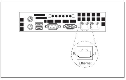
Figure 3-6. Ethernet Connector Location and Pinout
